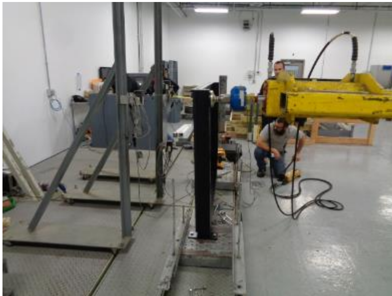
Photo No. 5 Concentrated Load Test at Top of Post
