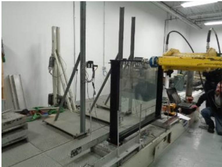
Photo No. 3 Concentrated Load at Top Rail Midspan
