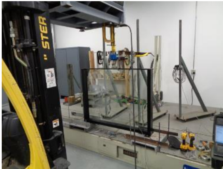
Photo No. 4 Concentrated Load at Midspan of Top Rail (Vertical)
