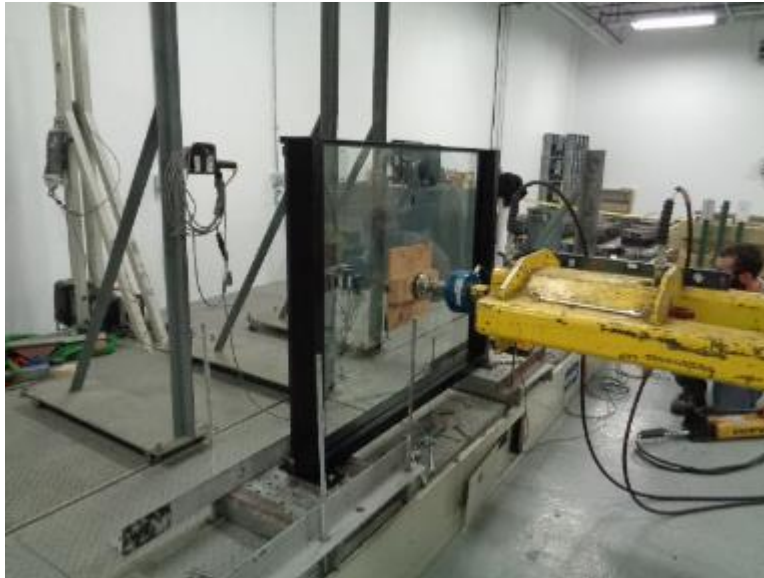
Photo No. 2 In-Fill Load Test at Center of Infill (Midspan)
